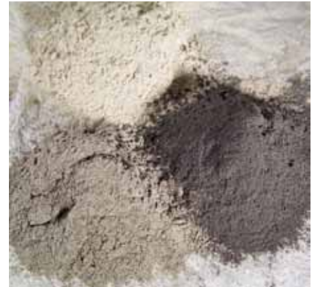
Figure 8a Fly ash, a byproduct of the electric industry, can be used as a partial replacement for portland cement. (Courtesy Portland Cement Association)
