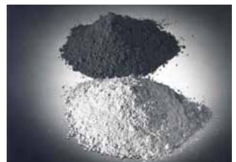
Figure 8c Silica fume, an industrial byproduct, is commonly used to replace cement in quantities from 5% to 7%. (Courtesy Portland Cement Association)
