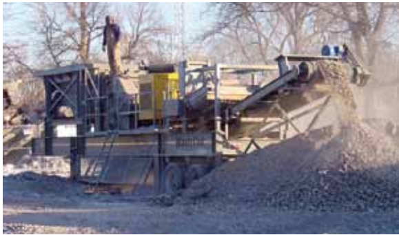
Figure 9 Crushed concrete from other sources can serve as recycled aggregate. (Courtesy Portland Cement Association)
